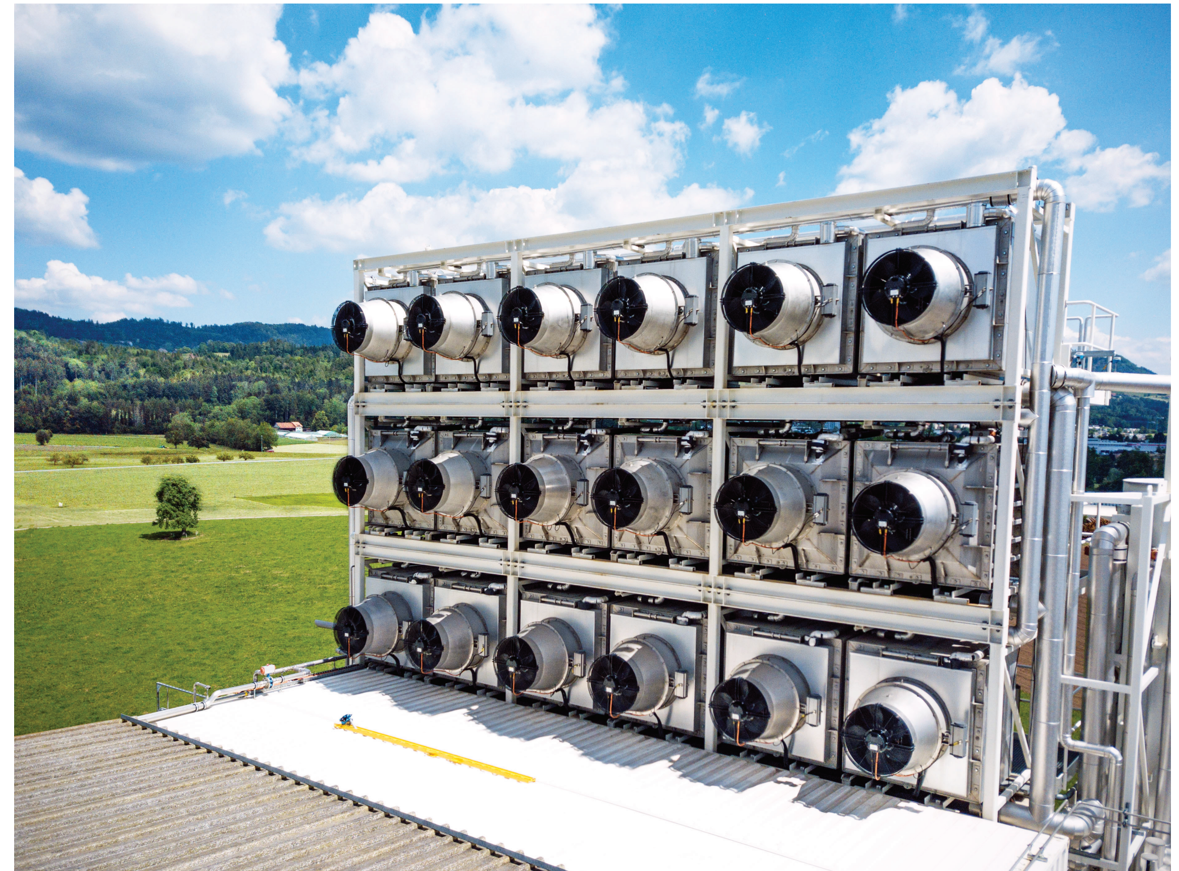
The Climeworks direct air capture technology runs exclusively on clean energy and the modular CO2 collectors can be stacked to build machines of any size. Source: Climeworks
