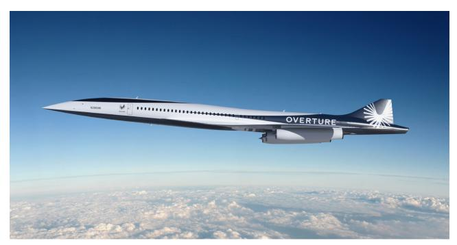
**Overture Milestones:** 2025 Rollout 2026 First flight 2029 Passenger flights Capacity: 65-80 passengers Sustainability: Net-zero carbon Cruising Altitude: 60,000 feet Routes: 600+ Length: 201 feet Wingspan: 106 feet Speed: Mach 1.7 Range: 4250 NM (4888 miles)
